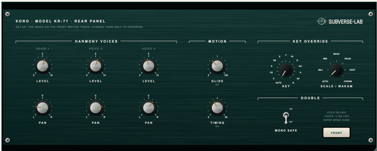
Rear plate (set-up panel). The front MOOD writes these; change them only to override it.
